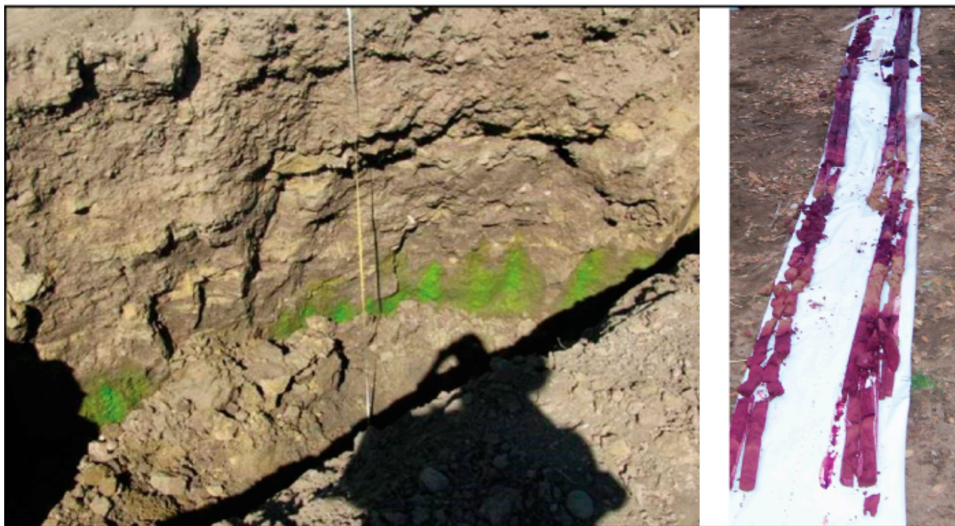
Figure 3-5. Heterogeneous and homogenous delivery of dye tracer.
